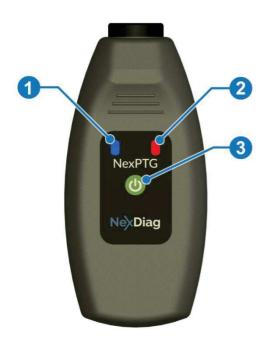
In order to start the **NexPTG** gauge the button 3 should be held down for three seconds until the power diode lights up on the panel 2 Next, start the **NexPTG** application on the mobile device (external). Correct communication will be signaled by the lighting up of the blue diode 1.
